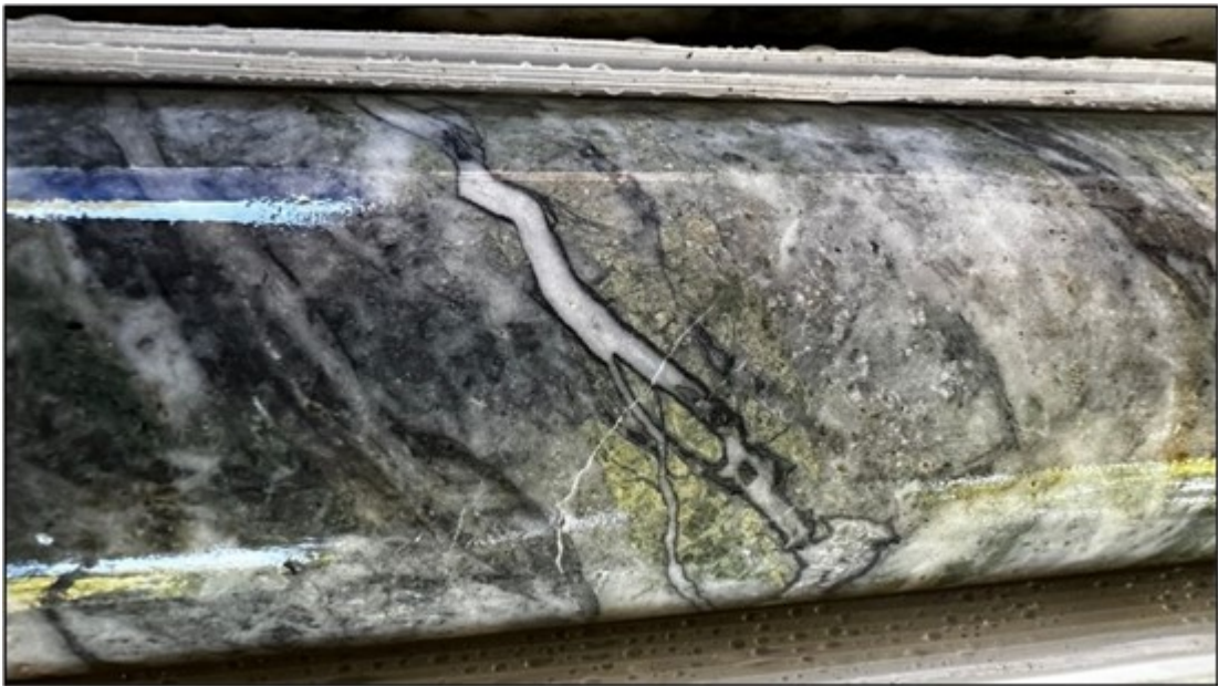
Details of core from hole PV-23-32 showing multistage mineralization. On the left, a vein with massive pyrite and chalcopyrite in gray quartz, cut by white quartz with a sphalerite margin. The right photo is a view looking at the end of the broken core. Assay results pending.
