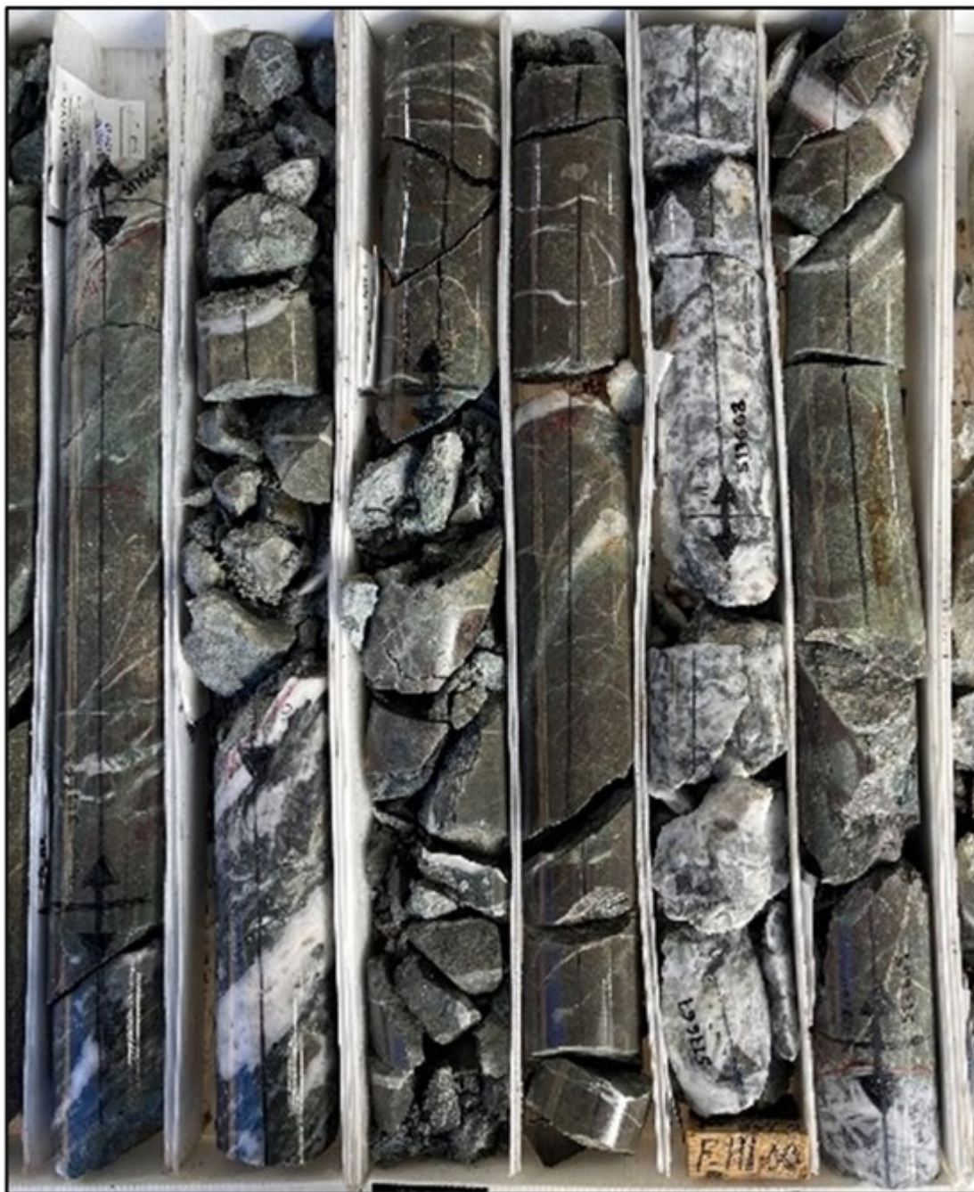
Photo of core from hole PV-23-32 showing intervals with multistage vein mineralization with brecciation and locally abundant sulfide minerals. Assay results pending.
