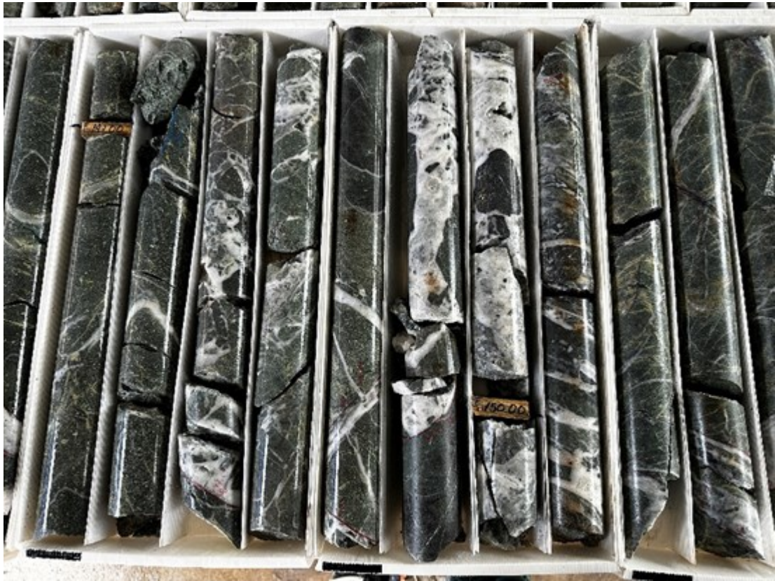
Photo of core from hole PV-23-32 showing intervals with multistage vein mineralization with brecciation and locally abundant sulfide minerals. Assay results pending.
