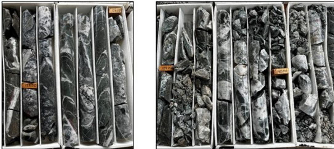
Photo of core from hole PV-23-29 showing intervals with multistage vein mineralization with brecciation and locally abundant sulfide minerals. Assay results pending.
