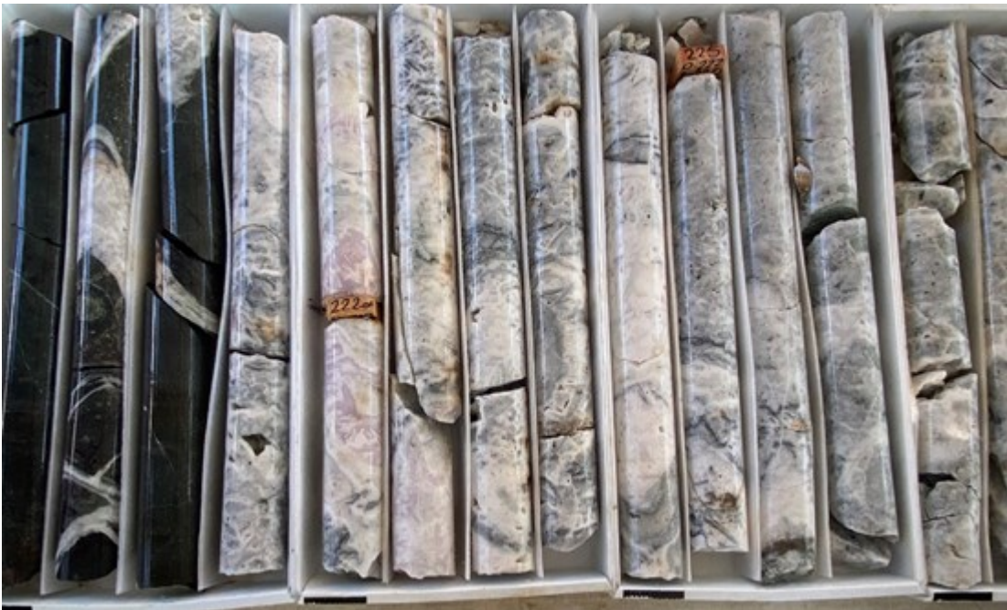
Hole #4 (PV-22-14) interval from 219.45 to 232.65, boxes 99 to 104, showing 9 meter wide multistage quartz vein in variably mineralized andesite.
