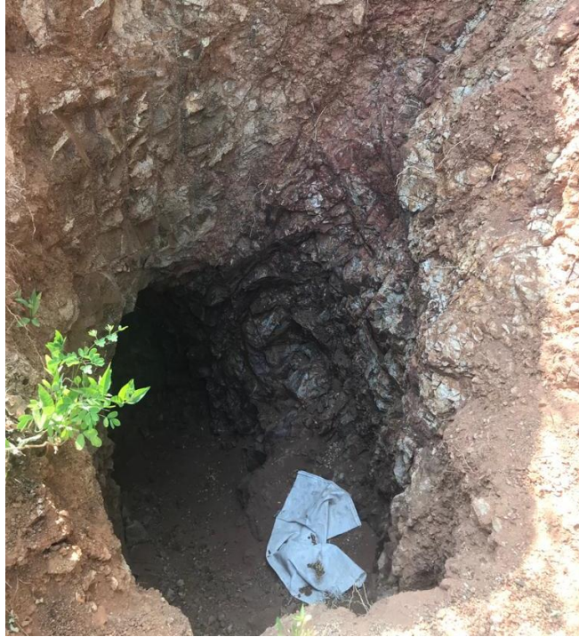
Figure 12.9. Photo of old working in Las Auras Area. Quartz vein and shear zone hosted in sericitized quartz-monzonitic intrusive.
