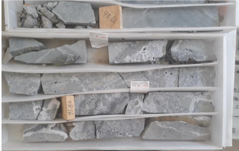
Figure 16.4. Core from the Palos Verdes Property. View of sample 13581; a coarse reject of this sample was assayed by the Author.
