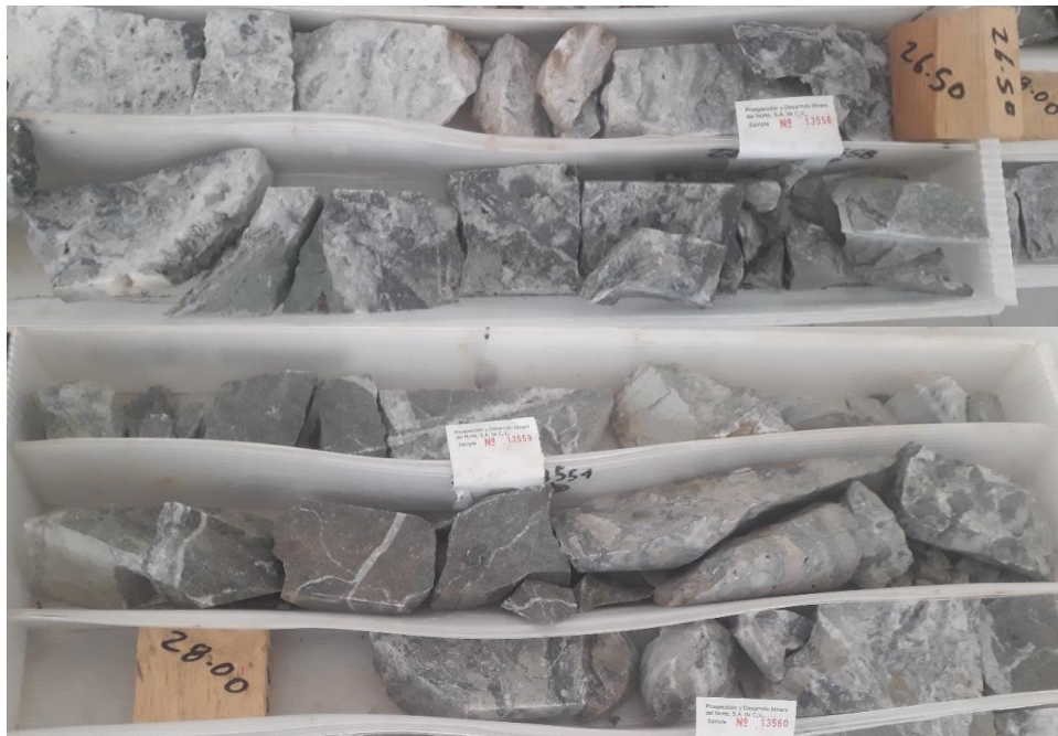
Figure 16.5. Core from the Palos Verdes Property. View of sample 13558 across two boxes; a coarse reject of this interval was assayed by the Author.
