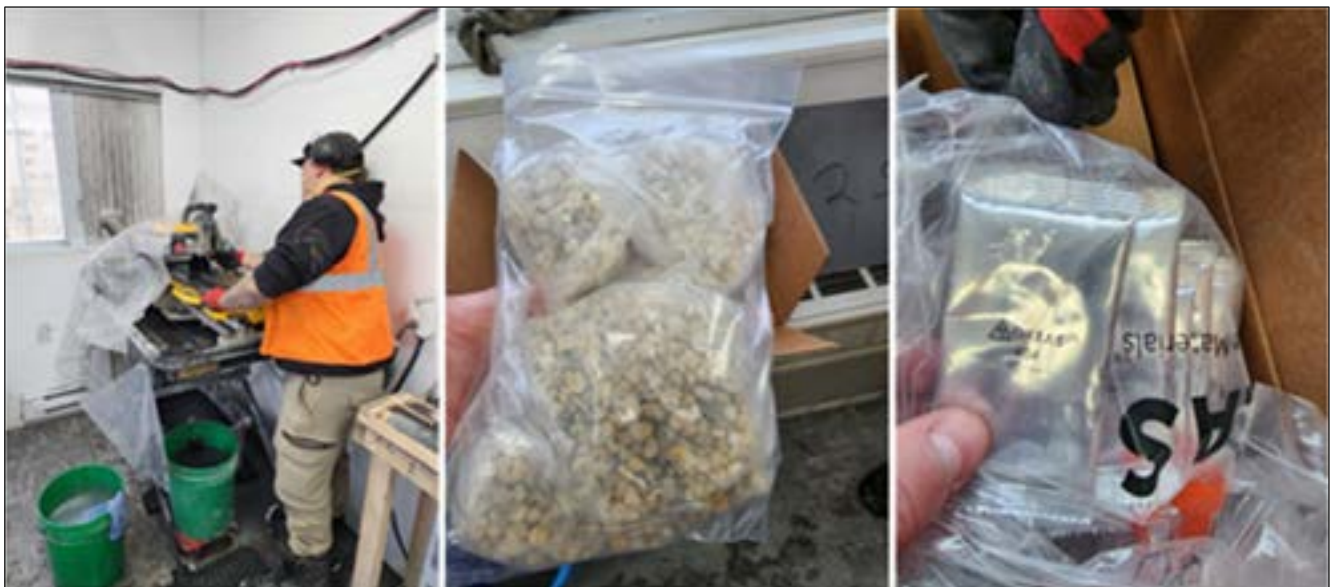
FIGURE 12-1 PHOTOGRAPHS OF CORE SAMPLING UNDERWAY AT MANOR'S FACILITY IN LA BAIE, SHOWING BLANKS (MIDDLE) AND CMRS (RIGHT) USED DURING THE 2022 DRILL PROGRAM
