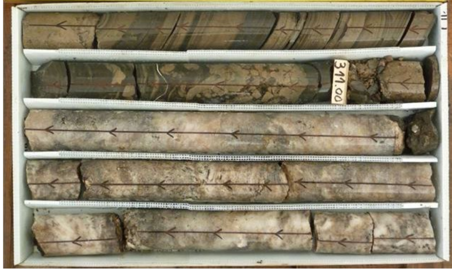
Figure 7-8: Massive borate mineralization in hole EVP2012-111 from 310.30 m to 313.20 m, situated at the contact between shale and dolomite units
