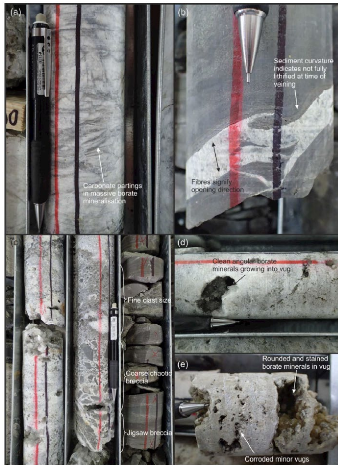
Figure 7-7: Mineralization textures: (a) Remnant carbonate partings in massive borate; (b) Layer-parallel vein showing vertical opening direction; (c) Variably brecciated interval; (d) Primary vug; (e) Secondary dissolution vug
