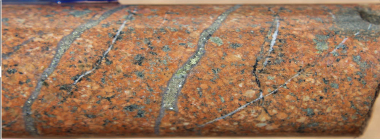
Figure 3: Duck Creek diamond drill core - Hole DCKDH016 – 398.50 metres. Hematite altered quartz monzonite with quartz-pyrite-chalcopyrite veining. Hole was drilled to a depth of 506.7 metres in an easterly direction (091°) with a dip of -70°.
