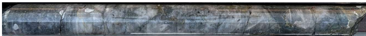
Figure 1: Drill core from hole CADH006, massive orogenic quartz vein with pyrite-pyrrhotite-marcasite-sphalerite-galena mineralization from 186.93 – 187.58 metres.
