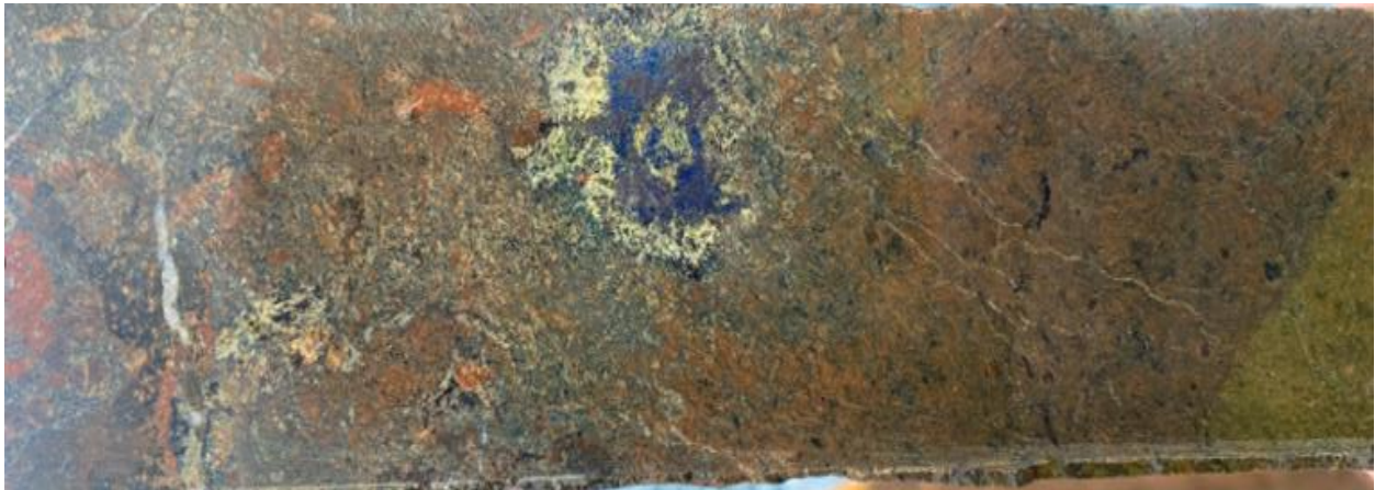
Figure 1: Hole DCKDH005 - ~395 metres – Drill core with blebs of bornite rimmed by epidote and carbonate hosted in feldspar-sericite-tourmaline-actinolite-pyrite altered volcanics.
