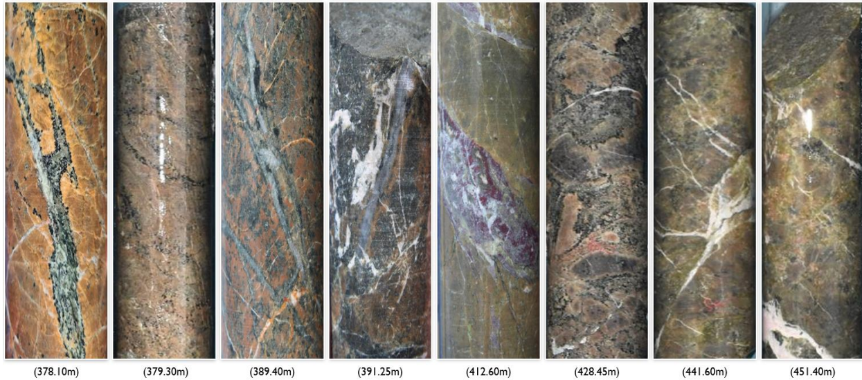
Figure 2: Drill hole DCKDH002 select core photos with interpreted geology. 378.10m – K-feldspar-actinolite altered volcaniclastic, 379.30m – biotite-magnetite-albite altered volcaniclastic, 389.40m – quartz-pyrite bearing B vein in K-feldspar-magnetite altered volcaniclastic, 391.25m – centreline quartz-pyrite B vein in biotite-albite-magnetite altered volcaniclastic, 412.60m – Sericite-carbonate alteration overprint on biotite-magnetite altered volcaniclastic cut by anhydrite veins, 428.45m – K-feldspar-magnetite-biotite breccia, 441.60m – biotite-magnetite with sericite-carbonate alteration overprint volcaniclastic, 451.40m – sericite alteration overprint on biotite-magnetite altered volcaniclastic.
