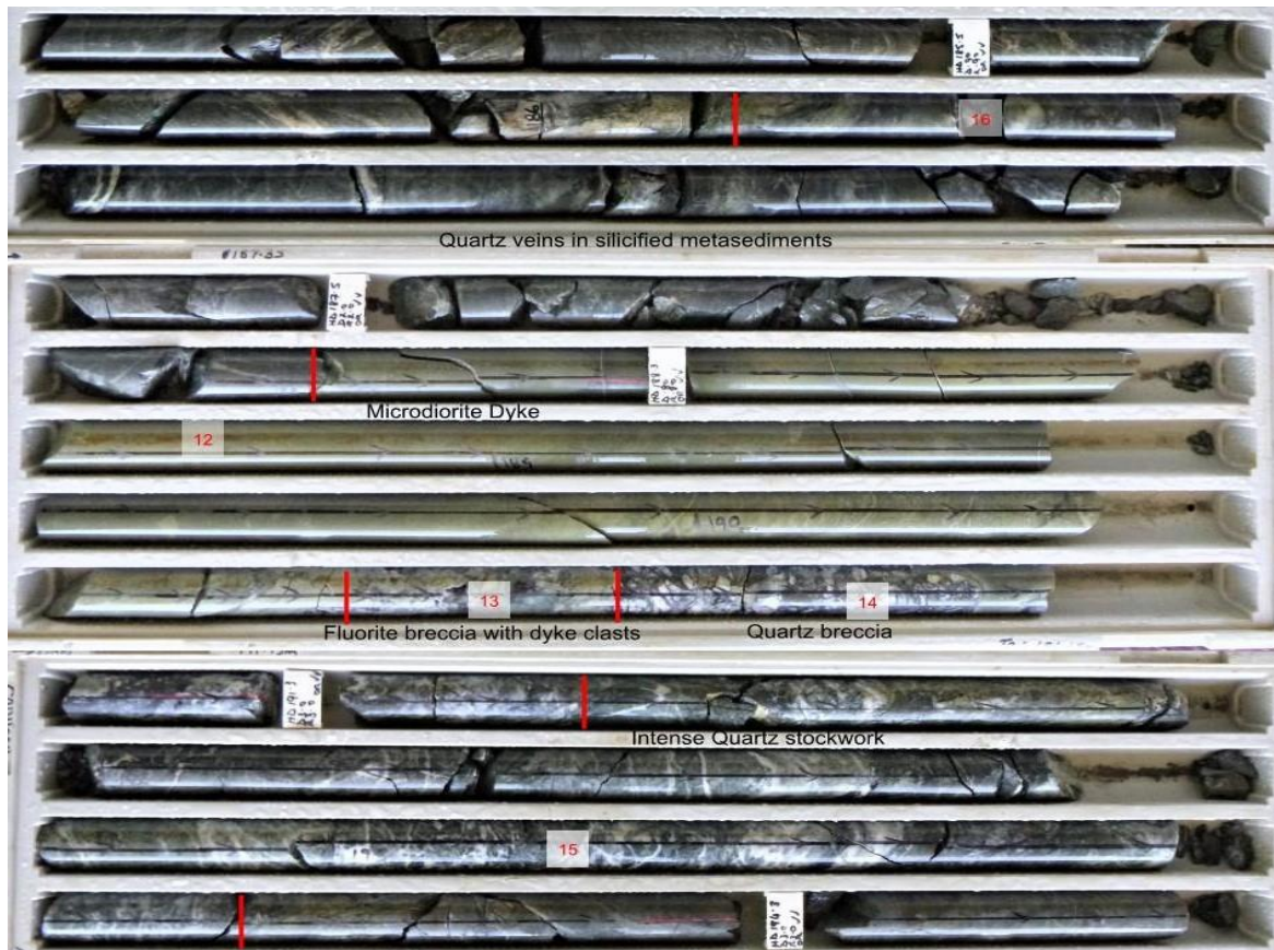
Figure 2 – CADH004 – Quartz veining and quartz vein stockwork extending from approximately 186.2 to 193.8 metres down hole.
