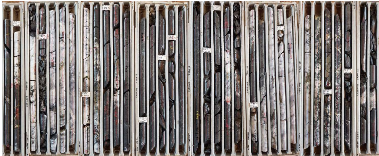
Figure 3 - Drill hole CADH002 ~183m to 206m - Interval of highly fractured psammities with a series of quartz veins and milled quartz breccias characteristic of the Croydon district.
