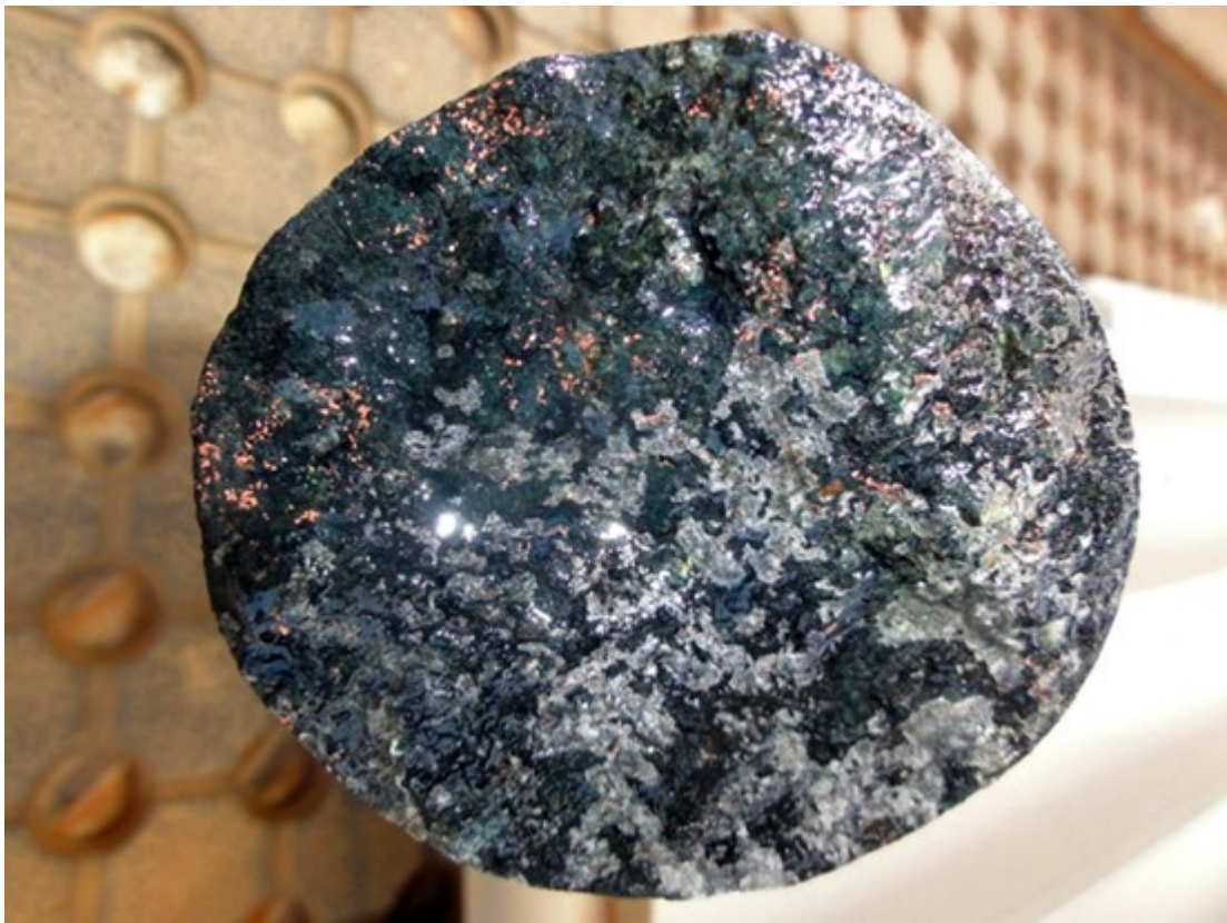
Figure 4: Drill hole MELDH001 - 250.30 metres - Native copper occurring on fractures.
