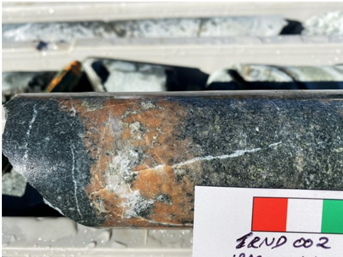
Figure 4: Photo of core from TRNDH002 (196.80m) showing pervasively chlorite-magnetite altered basalt with a crosscutting orange albite-quartz-carbonate-epidote-chlorite-pyrite-chalcopyrite vein.
