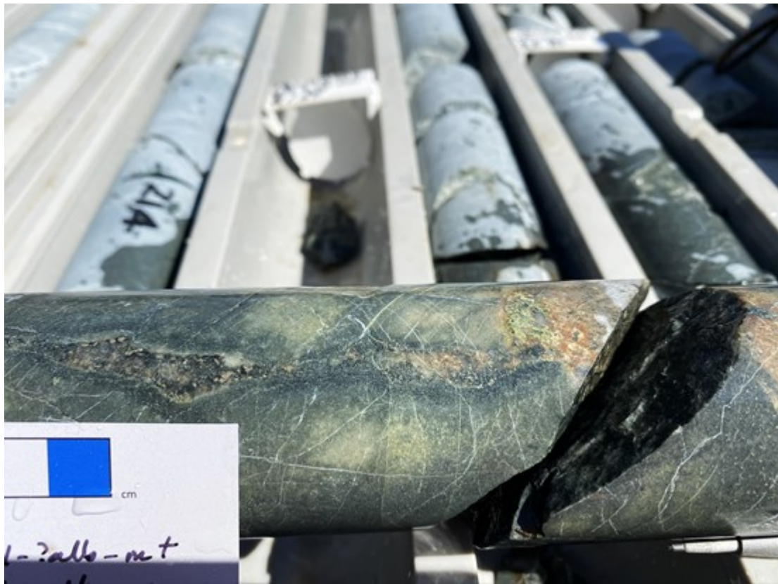
Figure 2: Photo of drill core from TRNDH002 (213.30m) showing complex multiphase alteration and veining associations. Early pervasive chlorite-albite-magnetite alteration overprinted by strong albite-epidote alteration further crosscut by complex quartz-epidote-albite-magnetite-chlorite-pyrite-chalcopyrite veins.
