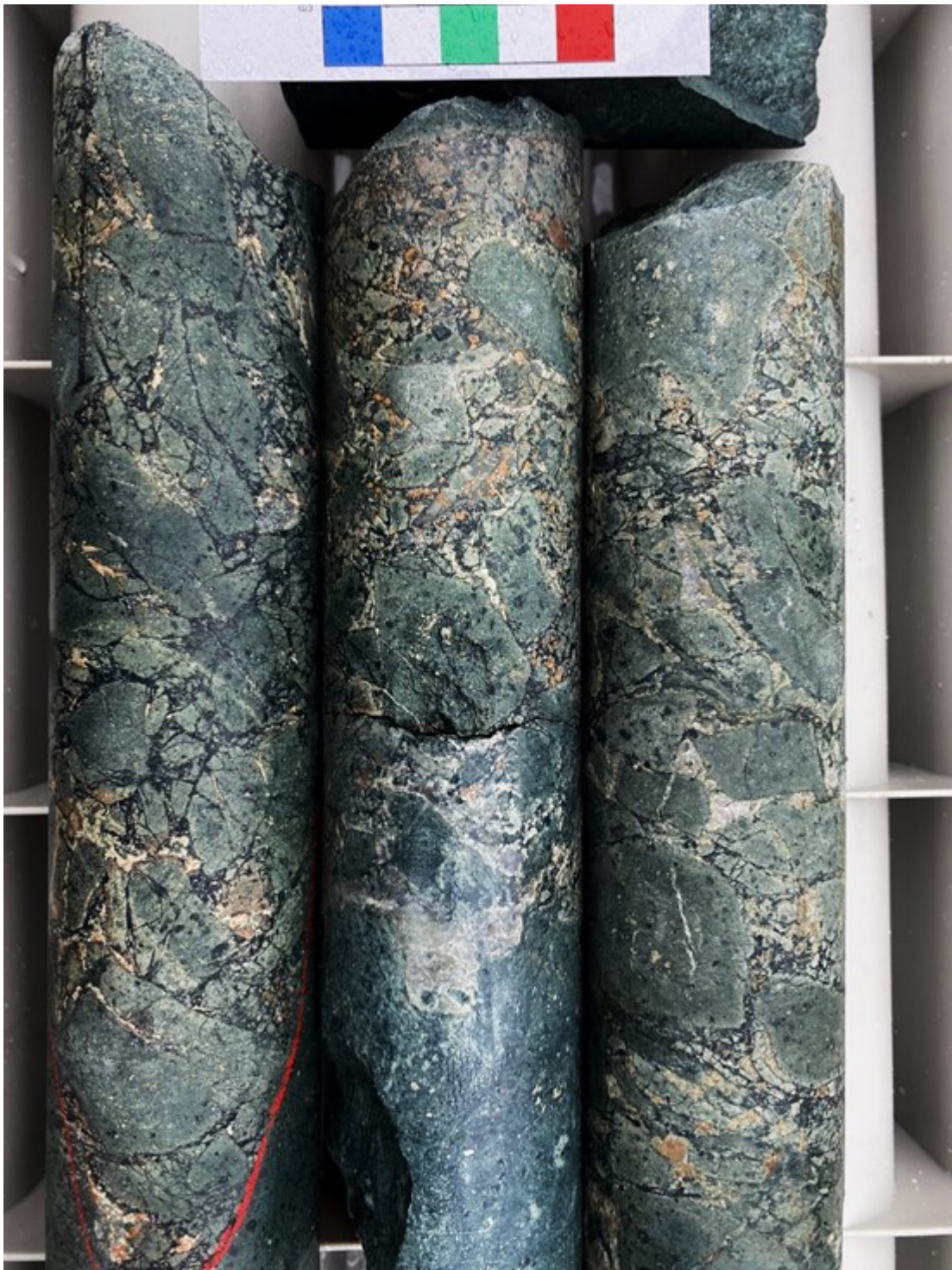
Photo 3. Nine Mile drill hole MYLDH001 183.5, 186.2 and 188.4 meters. Quartz-carbonate-chlorite cemented hydrothermal breccia. Breccias such as these are definitive indicators of hydrothermal fluid flowzones and are considered encouraging signs from a first-pass drill program.
