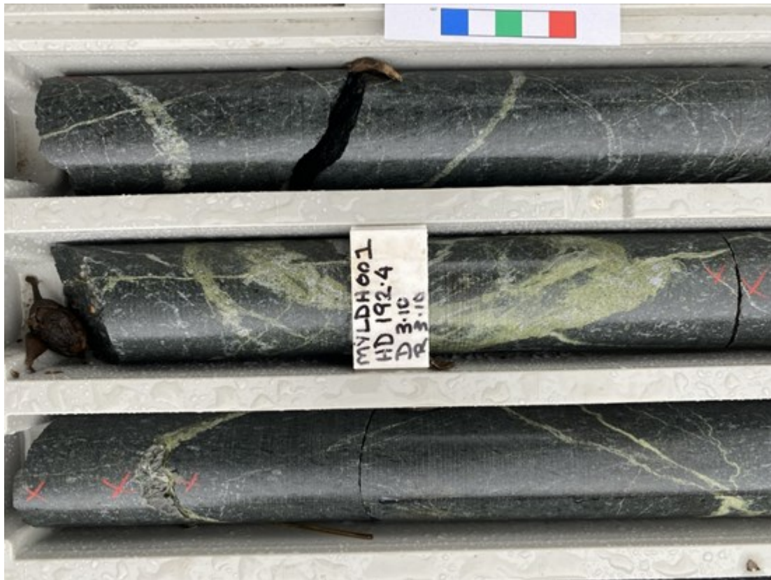
Photo 2. Myallmundi drill hole MYLDH001 192.40 meters. Close up of strongly biotite-magnetite altered basalt crosscut by quartz-carbonate and epidote-quartz-carbonate veins
