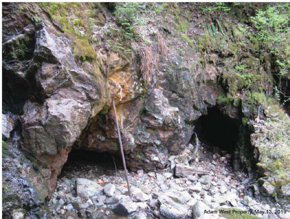
Figure 27. Lucky Jim adits on the east bank of the Adam River. Photos shows the portals to a short adit across the strike of the orangy rusted skarn mineralized layer on the left and a longer adit on the right that follows the mineralized dyke. A 5 foot steel bar rests against orange weathering calcareous precipitates above
