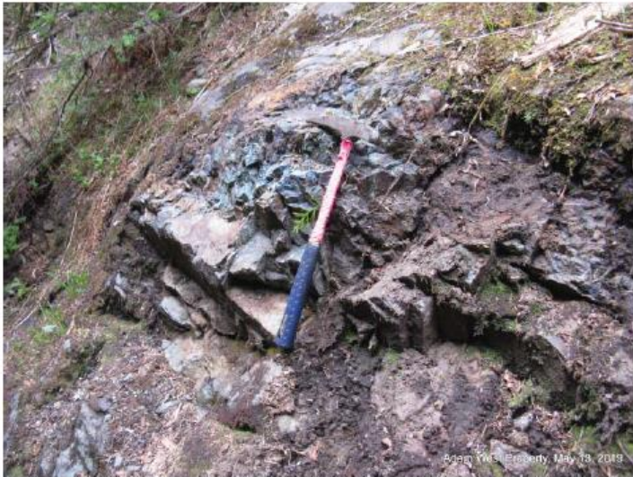
Figure 36. Massive bornite lens in altered volcanic rocks at Boyes Creek. The lens of bornite dips steeply to the right orthogonal to the hammer handle under the 20 cm of pink taped shaft. The lens continues for a few meters parallel to the hammer head. The sample at this site HW1602 graded 41.6 % Cu, and 145 g/t Ag.
