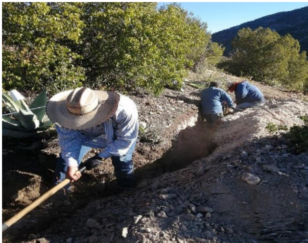
Photo 2A and 2B: Trenching and sampling in the Central Dyke Zone
