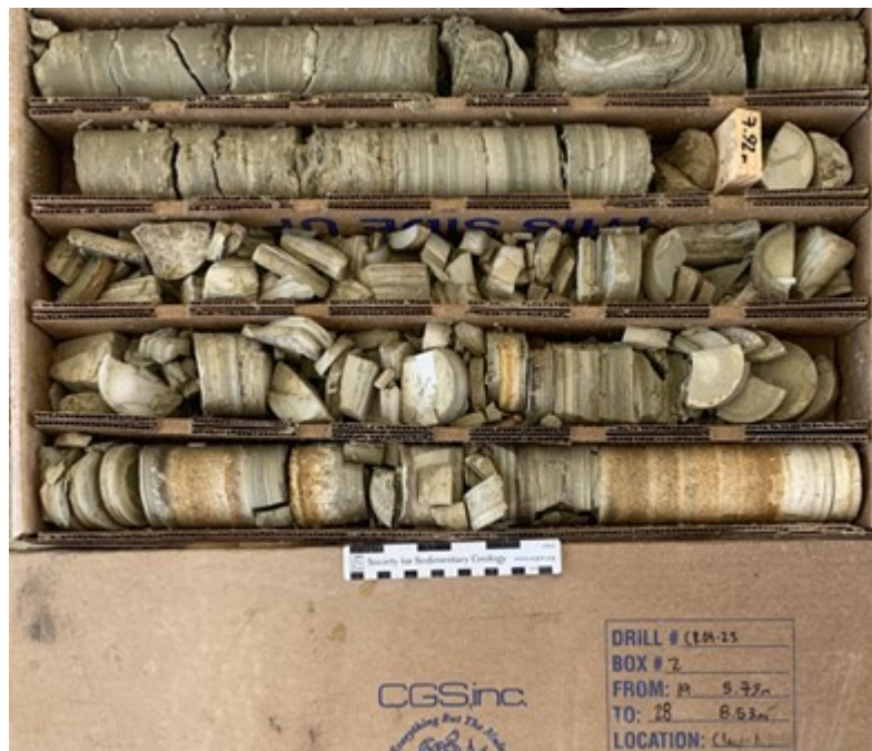
Photo #1: CR09-23 from 5.8-8.5 meters Finely laminated claystone with fine-grained crystal tufts interbeds
