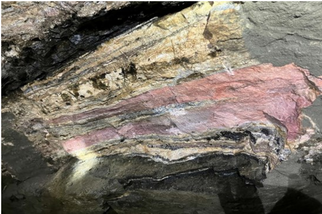
Figure 3. Photo of banded carbonatite about 4 feet wide composed of calcite (white), calcite + barite (yellow) + ancylite (pink); dark minerals are biotite and/or actinolite and possibly magnetite or allanite, Adit #3, right lateral.
