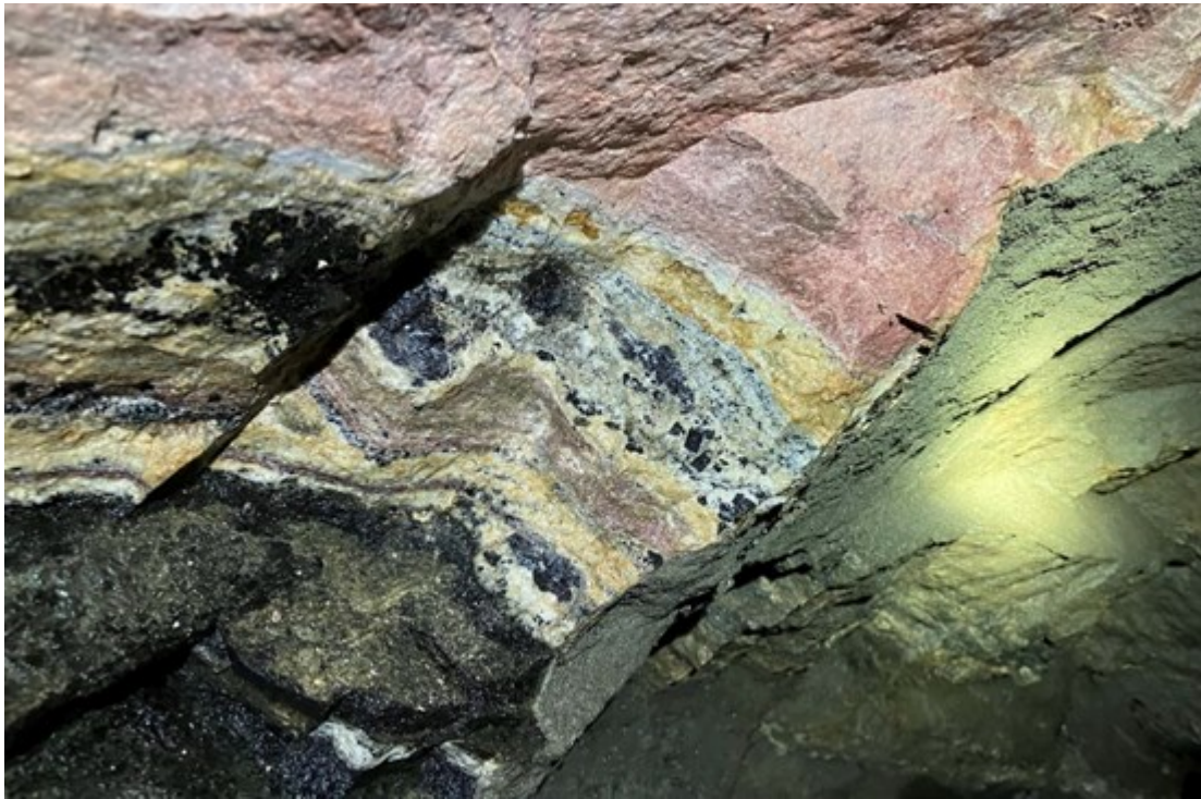
Figure 4. Photo of banded carbonatite composed of calcite (white), calcite + barite (yellow) + ancylite (pink) and monazite (honey colored); dark minerals are biotite and/or actinolite and possibly magnetite or allanite, Adit #3, right lateral.
