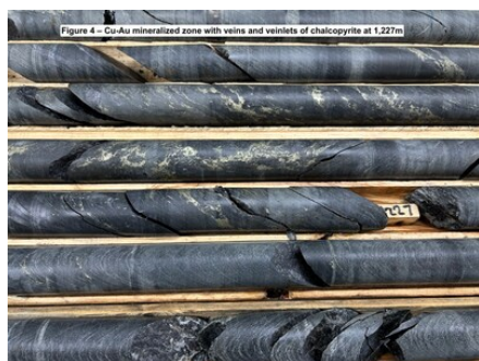
Figure 4 – Cu-Au mineralized zone with veins and veinlets of chalcopyrite at 1,227m
