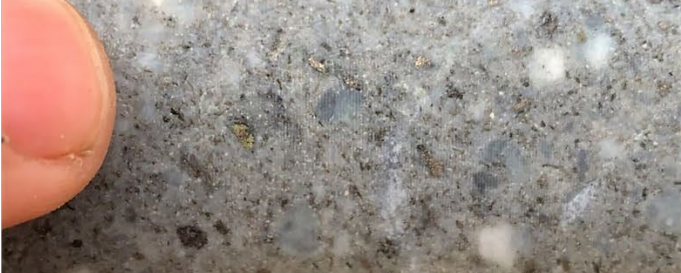
SLM22-011 – Quartz Diorite Porphyry Dyke with Disseminated Po-Cpy-Py at 337.00m.
