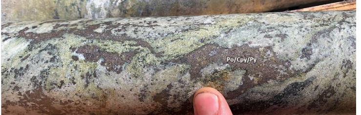
SLM22-011 – Massive Carbonate Replacement Sulphide (Py-Sph-Gn-Cpy) at 62.00m.
