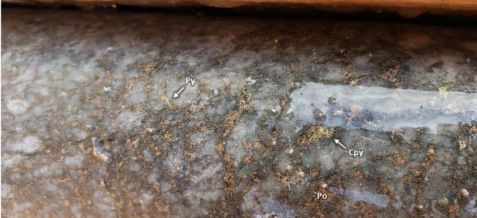
SLM22-011 – Quartz Diorite Porphyry Dyke with Disseminated Po-Cpy-Py at 337.00m.
