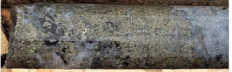
SLM22-011 – Massive Carbonate Replacement Sulphide (Py-Sph-Gn-Cpy) at 62.00m.
