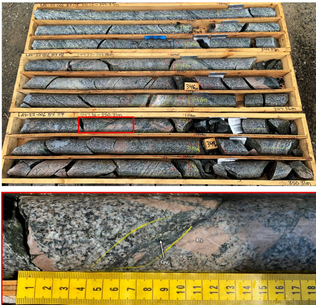
Figure 2: Photographs of HQ-sized core intervals from LAV22-006 showing increasing chlorite-magnetite±chalcopyrite and k-feldspar-dominant vein density near end of hole, hosted in variably altered granodiorite-to-diorite.
