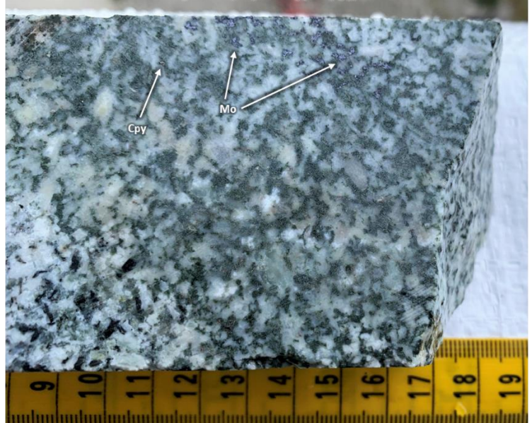
Figure 1: Photographs of HQ-sized core intervals from LAV22-006 showing Cu-Skarn and Cu-Mo porphyry style mineralization.
