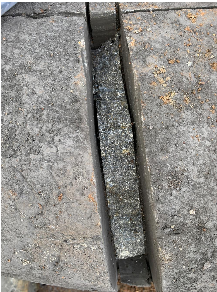
Figure 3. Sample 151608 collected during phase two program with visual estimates of 20-25% sphalerite, 15-20% pyrrhotite, 10-15% pyrite and 10% galena
