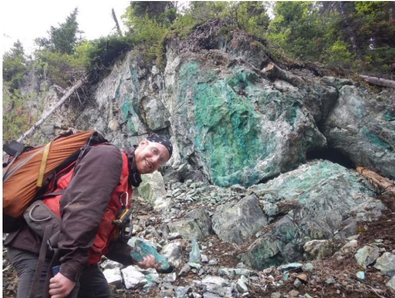
Figure 12-2. Mineralized outcrop exposure with a malachite rind on weathered surface
