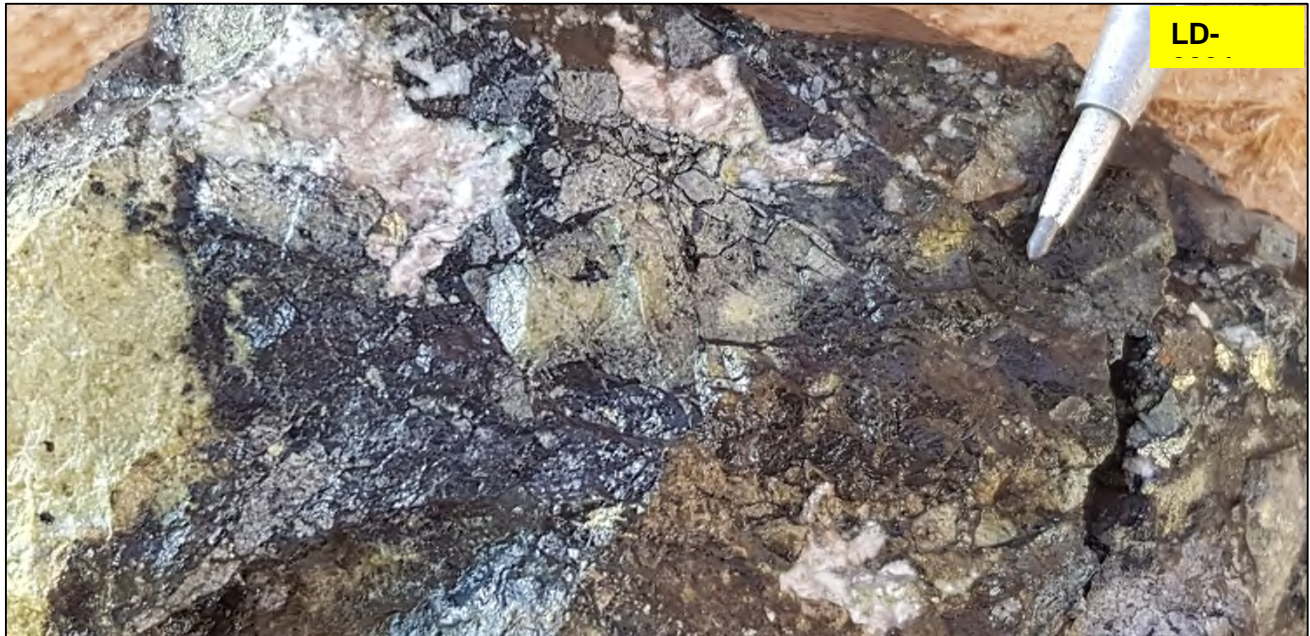
Figure 4. Poorly sorted; matrix-supported breccia with angular clasts of epidote and illitic clays set in a black, weakly magnetic matrix. Chalcopyrite as clast and as part of the matrix.
