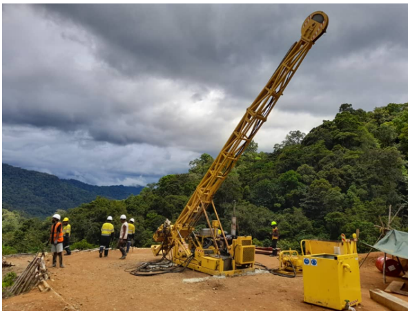
CS1000 drill on drill pad location of initial holes
