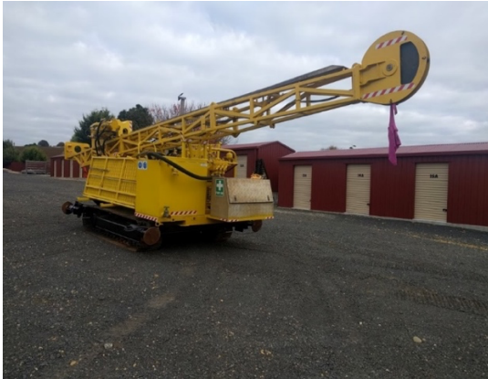
CS 1000 drill rig in Tasmania, Australia on tracks
