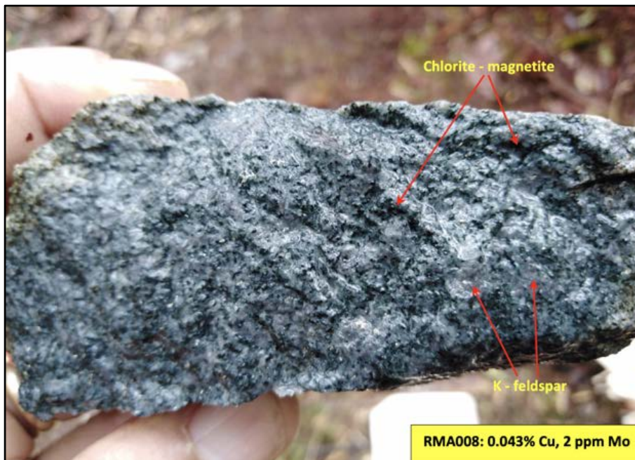
Photo 4: Selective rock outcrop sample of diorite, chlorite altered with disseminated magnetite and groundmass of k (potassium) - feldspar, 1-2% disseminated pyrite + chalcocopyrite. The selected sample above is not representative of the mineralization hosted on the property.
