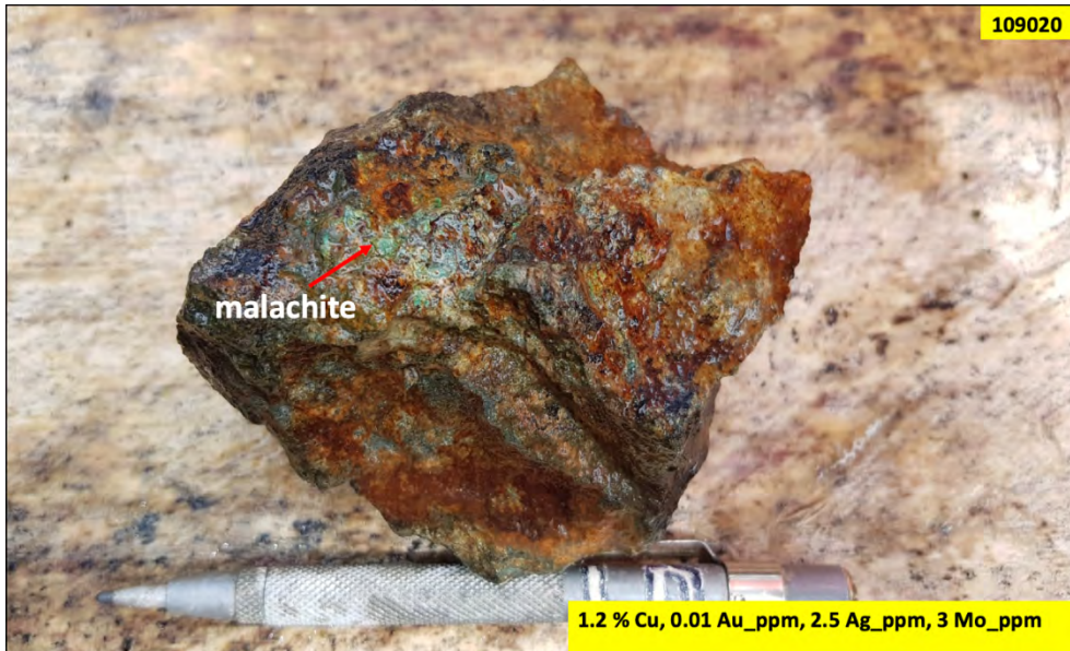
Photo 9: Selective rock sample from in situ outcrop of quartz – epidote - chalcopryite vein hosted by clay – chlorite - sericite altered diorite with malachite coatings.
