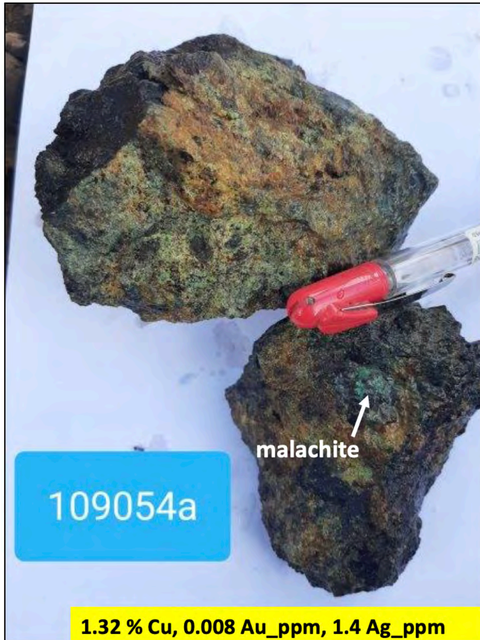
Photo 10: Selective rock float sample of microdiorite with malachite present as surface coatings and in fractures that also contain fine chalcopryrite.
