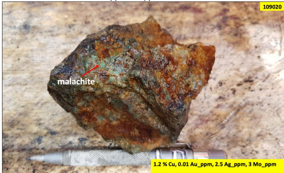
Photo 9: Selective rock sample from in situ outcrop of quartz – epidote - chalcopyrite vein hosted by clay – chlorite - sericite altered diorite with malachite coatings.
