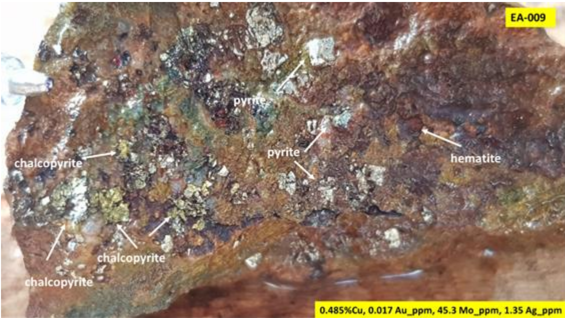
Figure A4: Grab sample from a transitional gossanous sub-crop of microdiorite with chalcopyrite and pyrite blebs/disseminations associated with hematite and limonite coatings.
