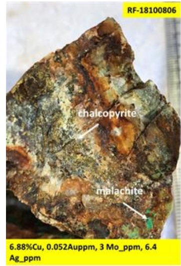
Figures A6, A7, A8: From left to right, Angular float sample of silicified and oxidized rock with pyrite and chalcopyrite associated with sericitic/clay alteration; Float sample in Omu Creek of quartz+chalcopyrite vein hosted by diorite with strong malachite coatings; Float sample in Omu Creek of limonitized rock with chalcopyrite and strong malachite coatings.
