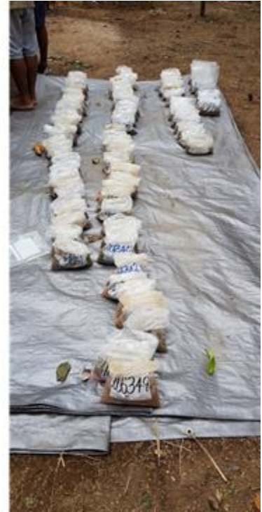
Figure A11: Geochemical soil sampling using hand auger (left), bagging of soil sample (centre), and sun-drying of soil samples prior to dispatch.
