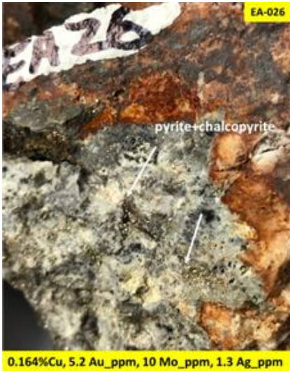
Figures A6, A7, A8: From left to right, Angular float sample of silicified and oxidized rock with pyrite and chalcopyrite associated with sericitic/clay alteration; Float sample in Omu Creek of quartz+chalcopyrite vein hosted by diorite with strong malachite coatings; Float sample in Omu Creek of limonitized rock with chalcopyrite and strong malachite coatings.
