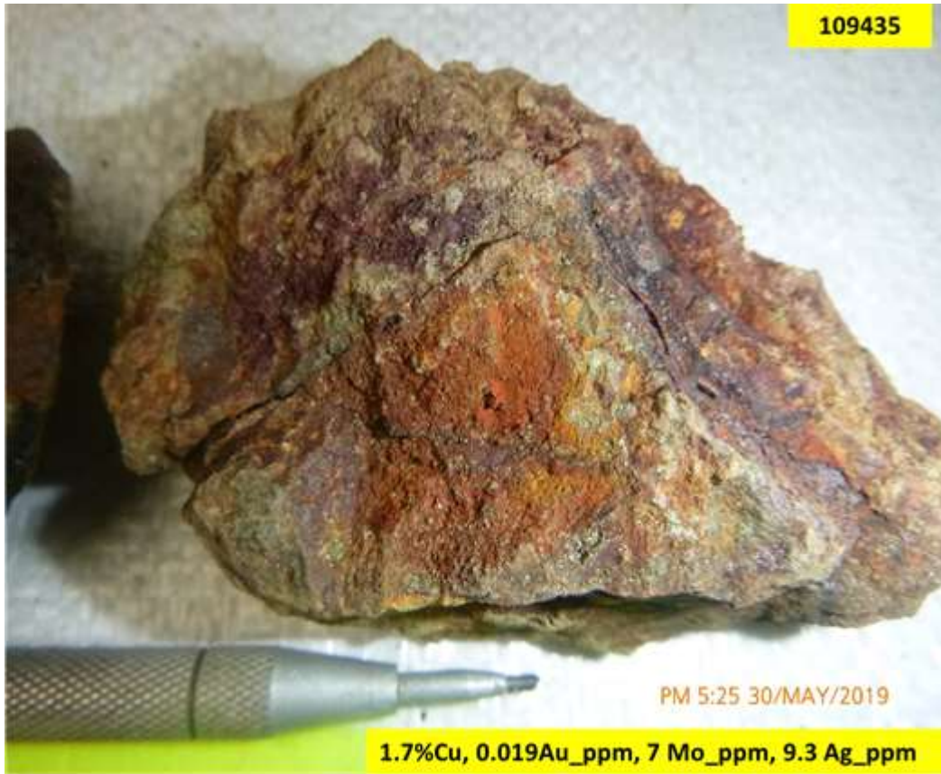
Figure A5: Grab sample from transitional gossanous outcrop of microdiorite with very fine disseminations of chalcopyrite and pyrite associated with limonite coatings.
