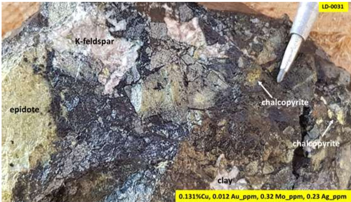
Figure A3: Grab sample from ~3m wide outcrop of poorly sorted hydrothermal breccia with angular K-feldspar, epidote and clay-altered clasts set in a weakly magnetic cement. Chalcopyrite as blebs/disseminations.
