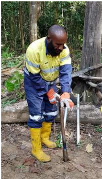
Figure A11: Geochemical soil sampling using hand auger (left), bagging of soil sample (centre), and sun-drying of soil samples prior to dispatch.
