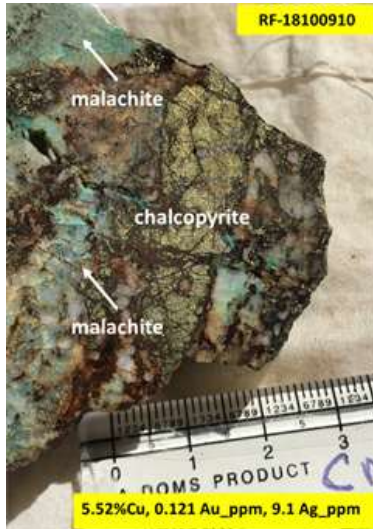
Figures A6, A7, A8: From left to right, Angular float sample of silicified and oxidized rock with pyrite and chalcopyrite associated with sericitic/clay alteration; Float sample in Omu Creek of quartz+chalcopyrite vein hosted by diorite with strong malachite coatings; Float sample in Omu Creek of limonitized rock with chalcopyrite and strong malachite coatings.
