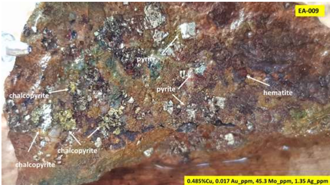
Figure A4: Grab sample from a transitional gossanous sub-crop of microdiorite with chalcopyrite and pyrite blebs/disseminations associated with hematite and limonite coatings.
