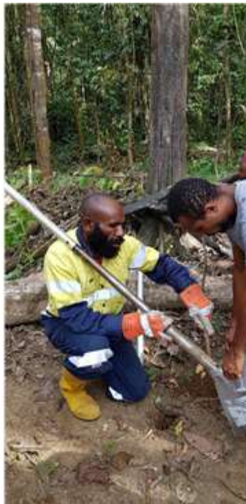
Figure A11: Geochemical soil sampling using hand auger (left), bagging of soil sample (centre), and sun-drying of soil samples prior to dispatch.
