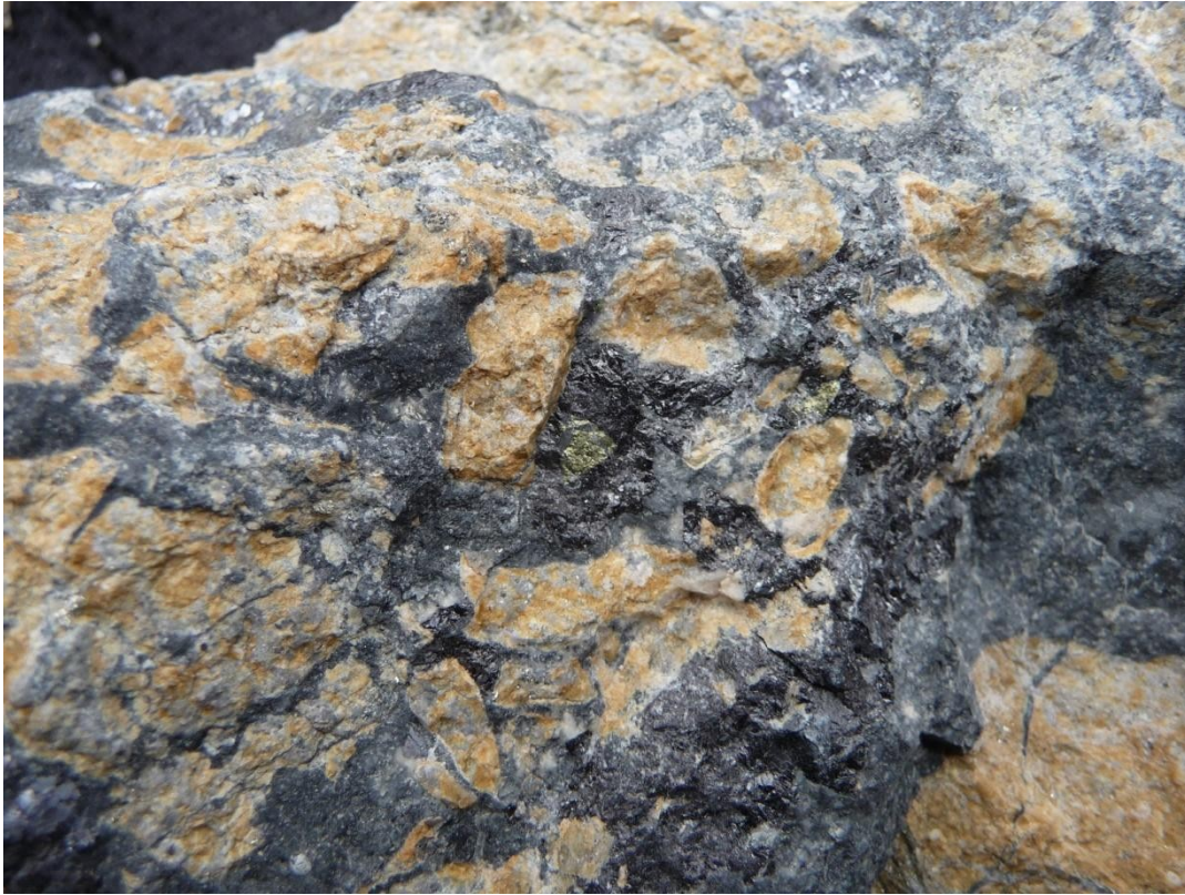
Figure 6.6: Clast supported breccia displaying angular to sub angular clasts
