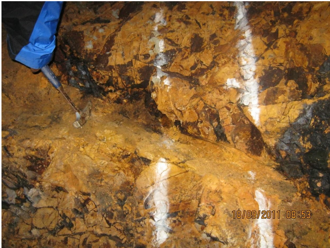
Figure 6.3: Rusty orange medium grained equigranular strongly altered dioritic rock
