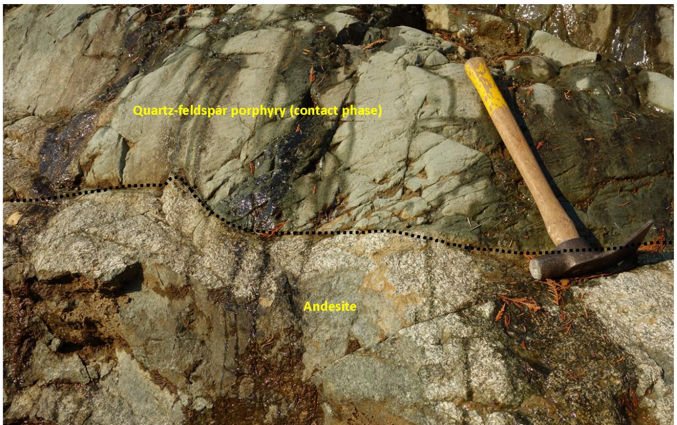
Photo 2-3 Contact between the quartz-feldspar porphyry (top) and the hornfelsed andesite within the potassic alteration zone with hammer for scale
