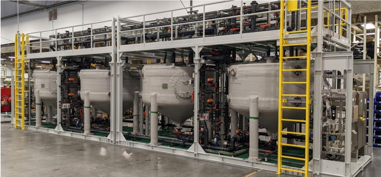
**Figure 17.6: Lithium Carbonate Reactor**
