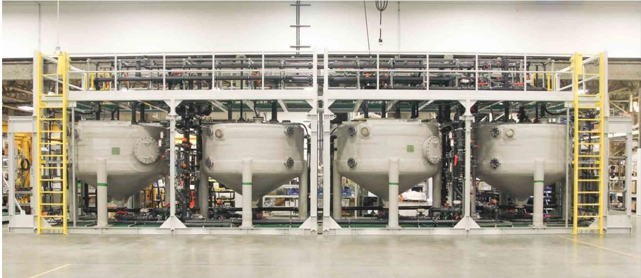
**Figure 17.4: Chemical Softening with Solid-Liquid Separation**
