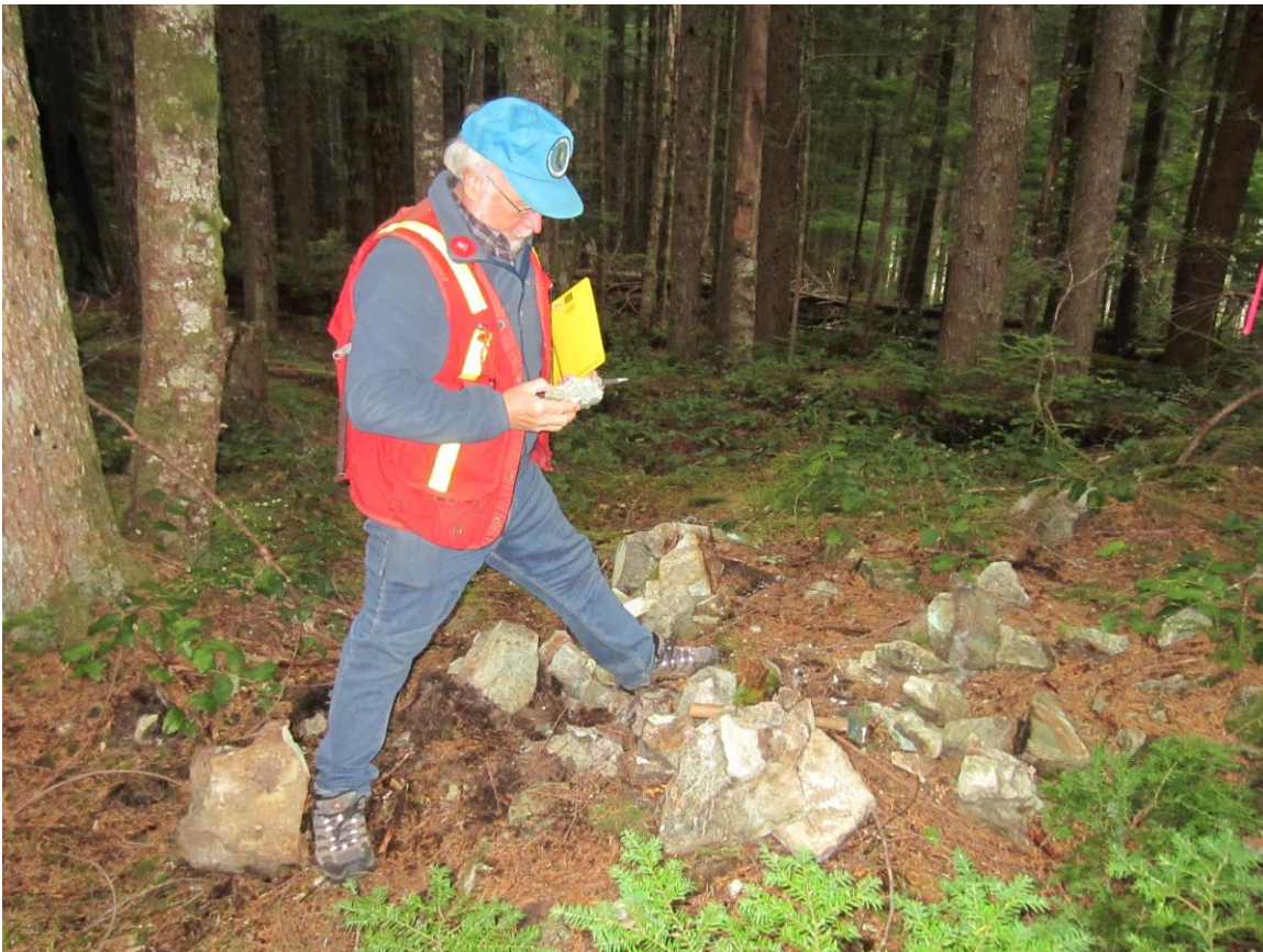
Photo 2. The author examining malachite stained granodiorite exposed in an old Rio Tinto exploration pit dating back to the 1970's (showing "C"). A sample collected at this locality in 2017 returned 5340 ppm Cu (Sample 30 - HM-17R30). Photo taken November 8, 2017.
