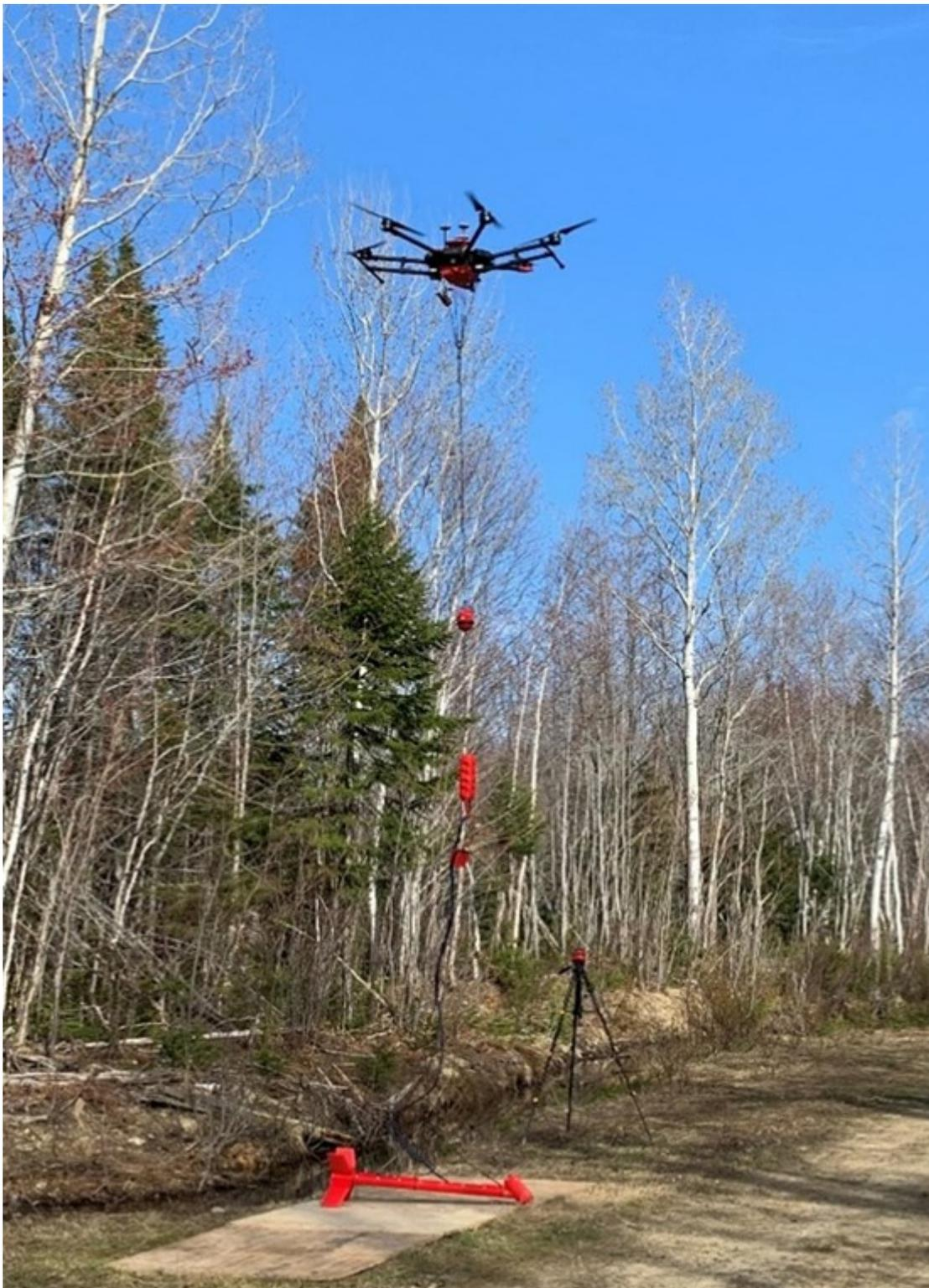
**Figure 3: UAV (Drone) and GPS Base Station**
