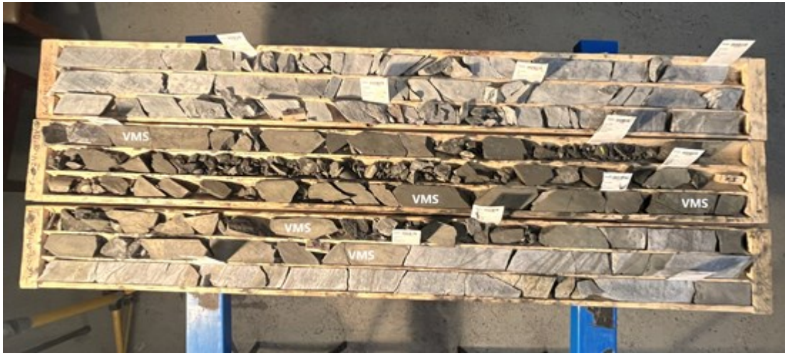
Figure 1: Pyritic VMS Mineralization in Drill Hole WD-24-01 at the Wedge Mine Project, Spanning 30.15 - 41.90 Meters of Depth
