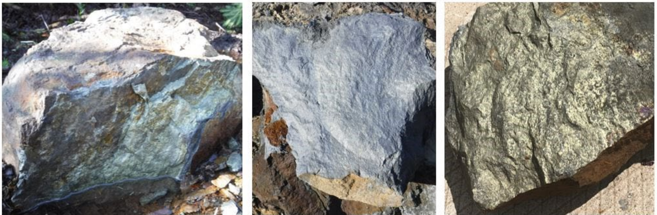
Figure 2: Massive Copper, Lead, Zinc, Silver, Gold Lens Ore, Nine Mile Brook Lens Bulk Sample
