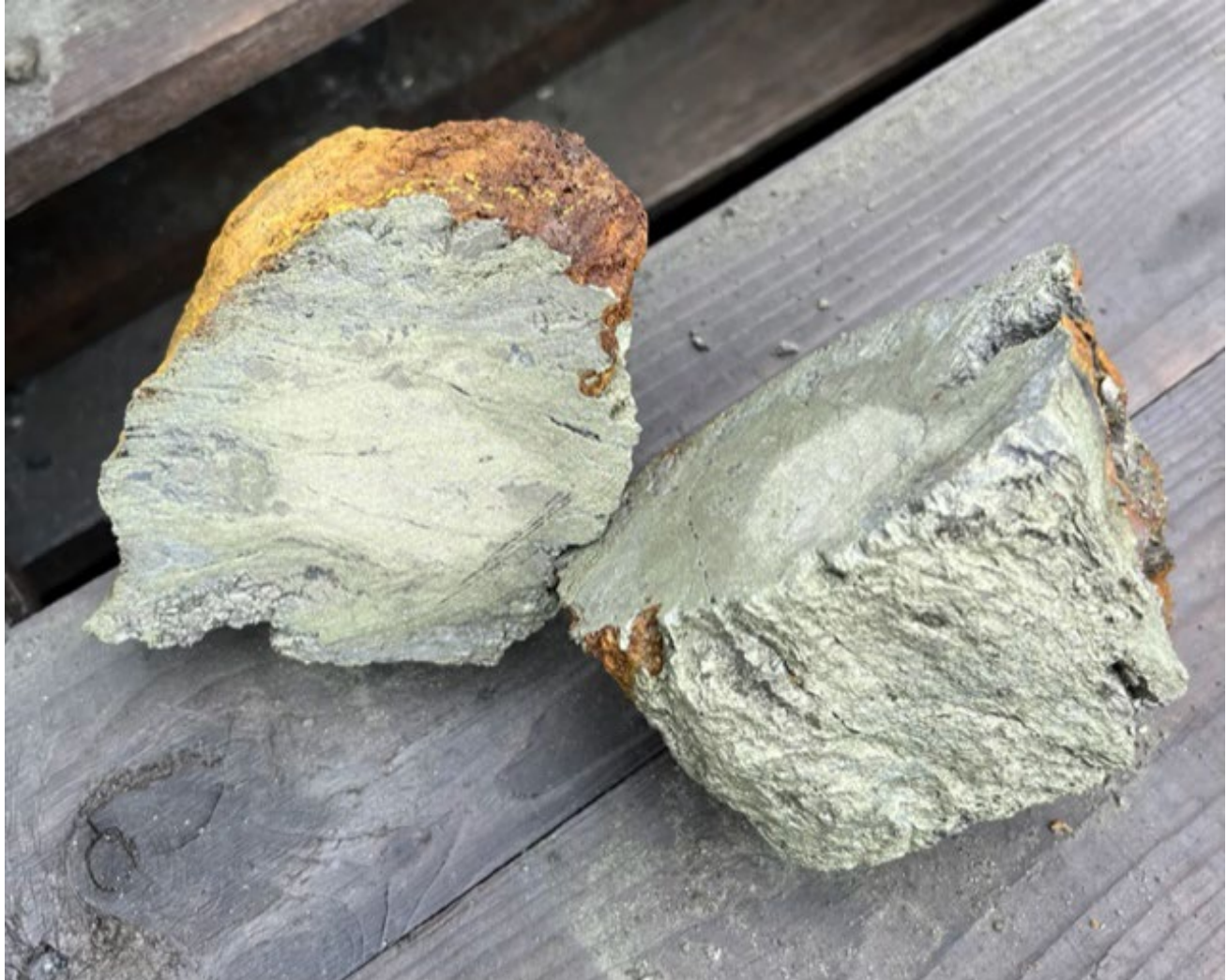
Figure 2: Wedge Sample #W23015 XRF Results (24.81% Cu, 0.20% Pb, 0.40% Zn) (Ag & Au TBD)
