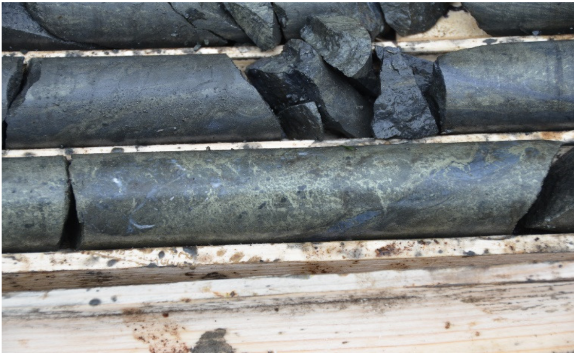
Massive VMS Mineralization – Chalcopyrite (Cu), Sphalerite (Zn), and Galena (Pb). Silver (Ag) and Gold (Au) to be determined.
