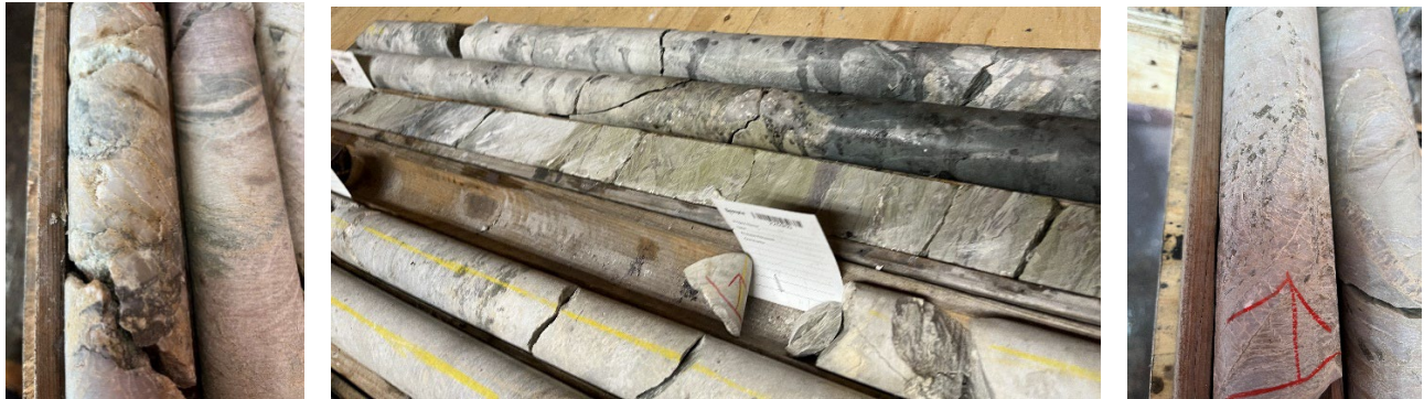
DDH - CL2203 -CL2205 (New Gold Target). Cut samples sent to ALS Global Laboratories for Fire-Assay Au.
