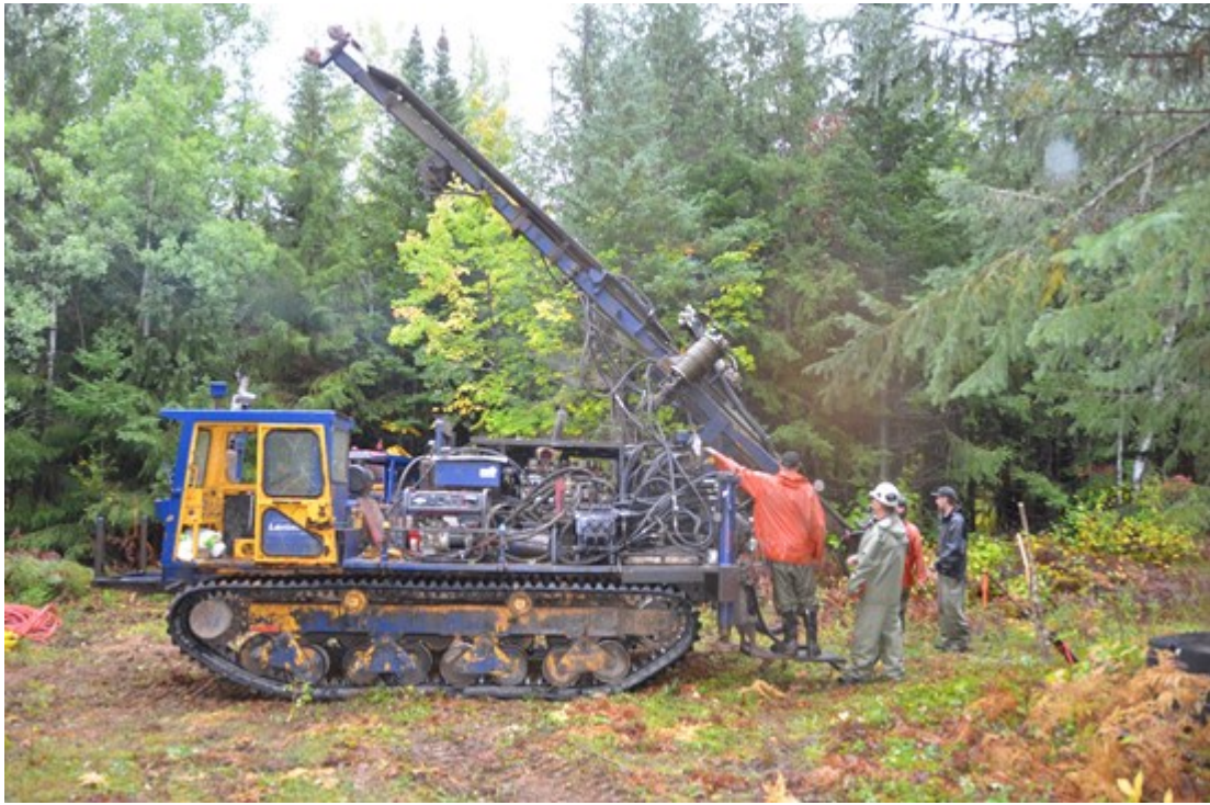
Figure 2: Environmentally Conscious Lantech Drilling Mini Track Mounted Diamond Drill Rig
