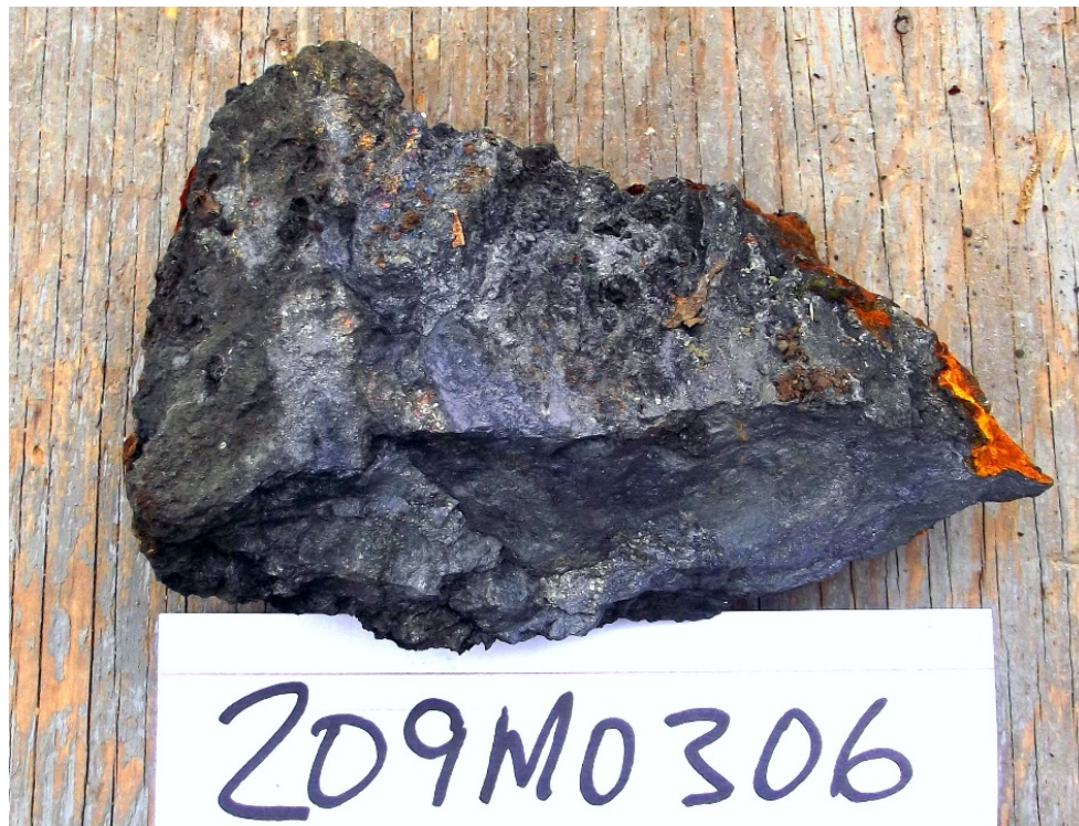
Figure 18: Massive, banded mineralization, >20% Pb, 19.73% Zn, 3.67 g/t Au, 217 g/t Ag.
