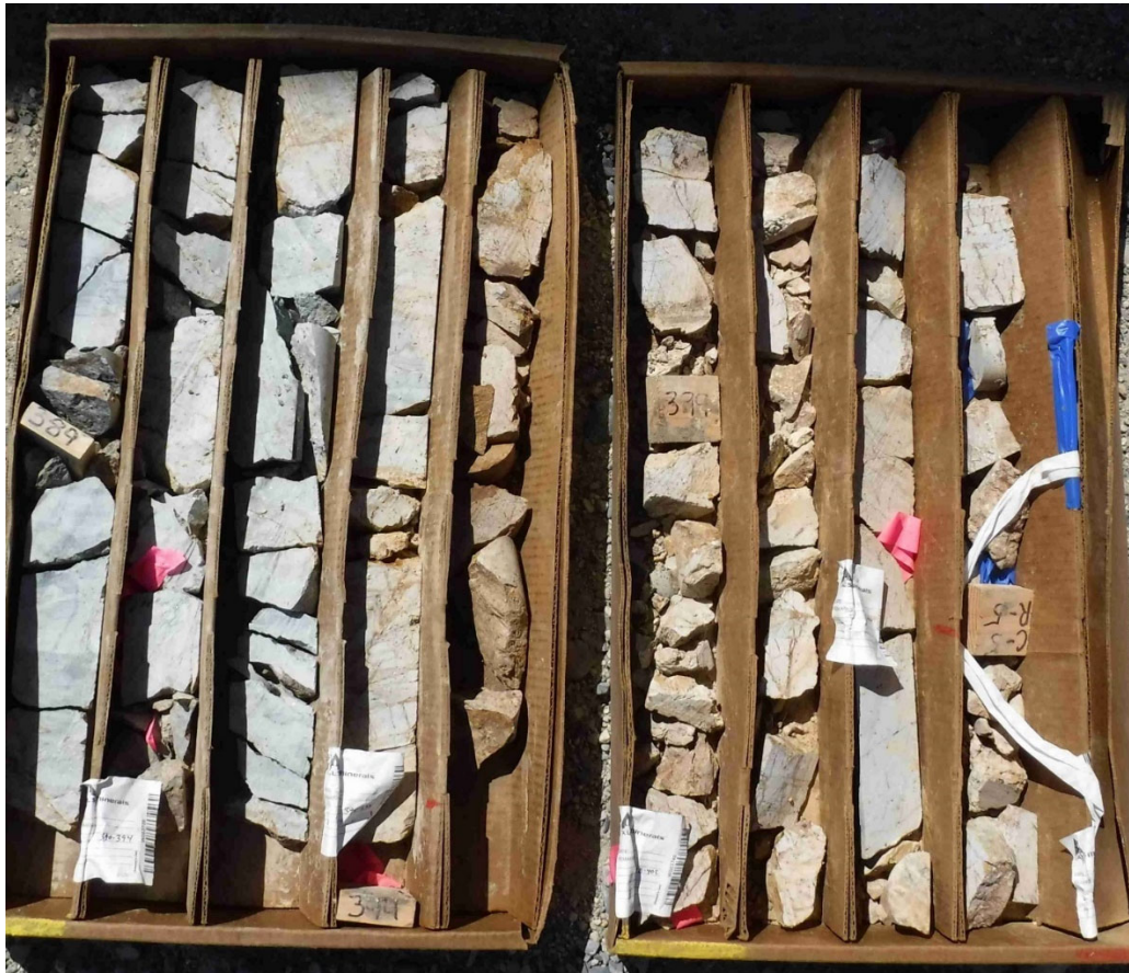
Figure 12-1 Drill hole CRR17-009, Wood Canyon Formation Mineralized Interval of Phyllite and Oxidized Quartzite (approximately 389 to 401 ft depth).
