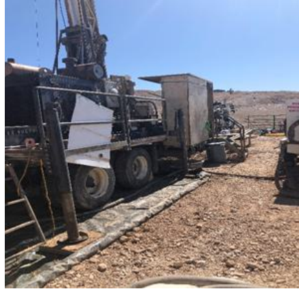
Figure 8-1: Truck Mounted Core Rig
