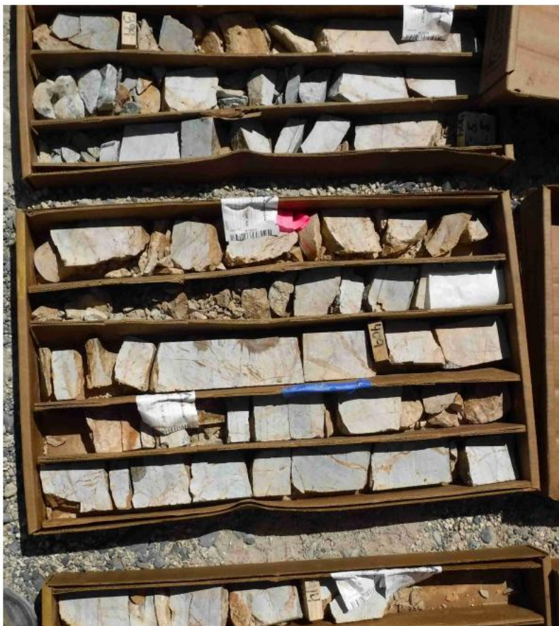
Figure 12.2. Drill hole CRR18-014, Wood Canyon Formation Mineralized Interval of Brecciated/Re-healed Quartzite and Sheared and Foliated Phyllite (approximately 399 to 414 ft depth).
