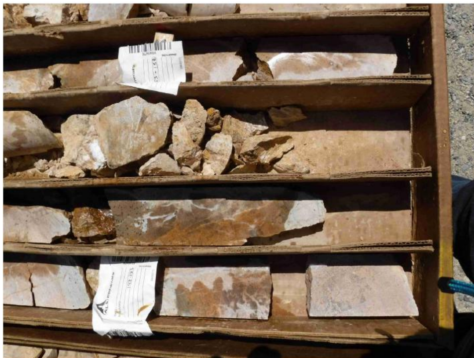
Figure 12.3. Drill Hole CRR18-024, Wood Canyon Formation Mineralized Interval of Quartzite (approximately 148 to 153 ft depth).
